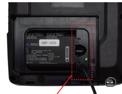
Connect the AC adapter to the main unit to charge the battery.
