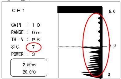
If STC value gets bigger more than necessary, the sensitivity of upper part of the ultrasonic reflection wave is reduced like the chart above, moreover, the whole sensitivity is also affected and reduced by STC value.
