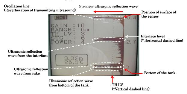
The ultrasonic reflection wave is displayed by graph.
