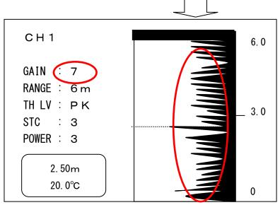
Next, in the chart below, there is a fear that it is impossible to distinguish the ultrasonic reflection wave from the interface as being different from others because the ultrasonic reflection waves from the upper part is too strong except the oscillation line. Therefore, set STC value to smaller value.
