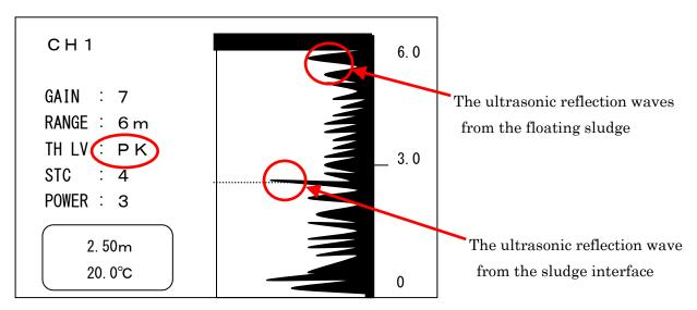
And then, set TH LV value as the ultrasonic reflection wave from the interface can always exceeds TH LV.
