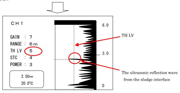
Optimize the settings to display the ultrasonic reflection waves like the chart below.
