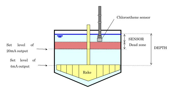
The distance within 0.4m from the surface of the sensor is dead zone; HL2000 can't measure this range at all.
